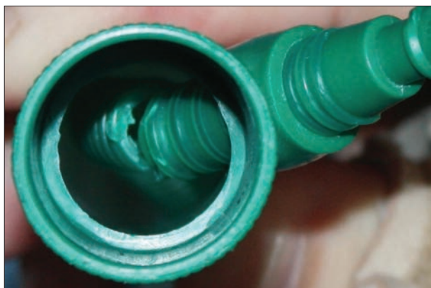
Figure 2—Photograph of the machine end of the Mapleson D breathing system with Bain coaxial adaptation used during anesthesia of the dog in Figure 1. Visual inspection revealed a tear in the inspiratory tube.
