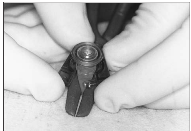
Figure 4—Positioning of the valve clip, which was snapped snugly over the tube and valve stem.
