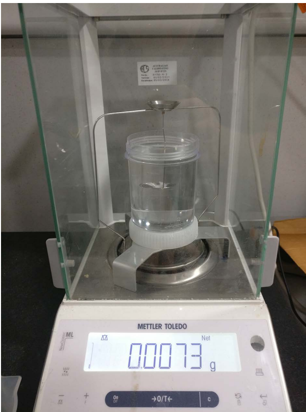
Figure 3 —Setup for suspension method of water volumetric analysis using Mettler Toledo microbalance. Sample pictured is a dissected nucleus pulposus suspended in distilled water on hydrostatic weighing scale apparatus. The weight of the nucleus pulposus is displayed in grams.
