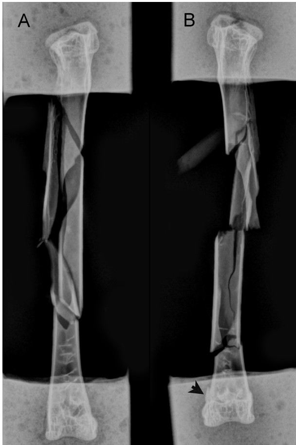
Figure 2 —Representative radiographic images of the tibiotarsal bones for one of the red-tailed hawks described in Figure 1 that were obtained after biomechanical testing to failure in torsion (A) and in compression (compression test; B). For the compression test, each bone was loaded in axial compression at 2 mm/s under actuator displacement control until the bone failed. Load and linear actuator displacement data were acquired at 128 Hz throughout the test. All bones that underwent the compression test developed a defect in the distal metaphysis (black arrow). See Figure 1 for remainder of key.
