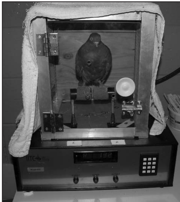
Figure 1—Photograph of an incapacitance meter modified for birds. For each measurement, domestic pigeons ( Columba livia ) were placed on a perch composed of 2 separated sections, each linked to a scale to measure weight bearing on each limb.
