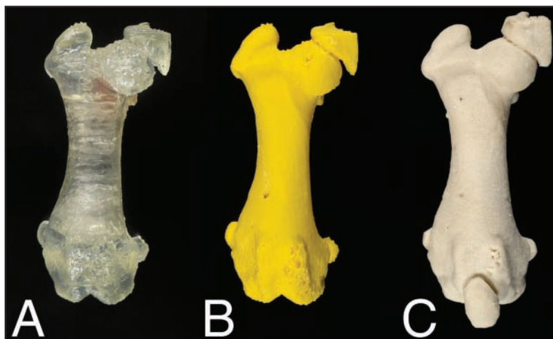
Figure 1—Photographs of biomodels of a canine femur made by use of SLA (A), FDM (B), and cyanoacrylate-impregnated plaster casting (C).
