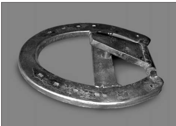
Figure 1—Photograph of a custom-made adjustable heart-bar shoe used to induce transient lameness in 17 horses. The screw in the straight bar is tightened to raise the heart bar and thereby put pressure on the frog of the horse's foot to create temporary lameness.
