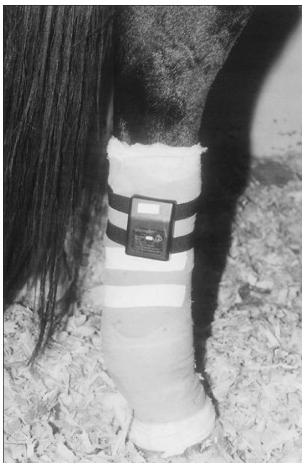
Figure 1—Photograph of step monitor placed over the third metatarsal bone for monitoring loading events.
