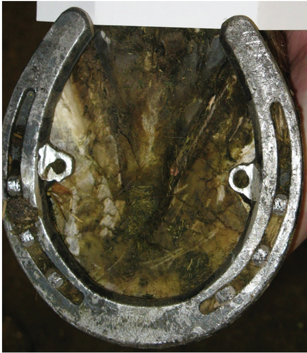
Figure 2 —Picture of the steel keg shoe with nuts welded onto the inner aspect of the medial and lateral branches of the shoe for insertion of screws, which were used to induce unilateral forelimb lameness grade 3/5 in the horses described in Figure 1.
