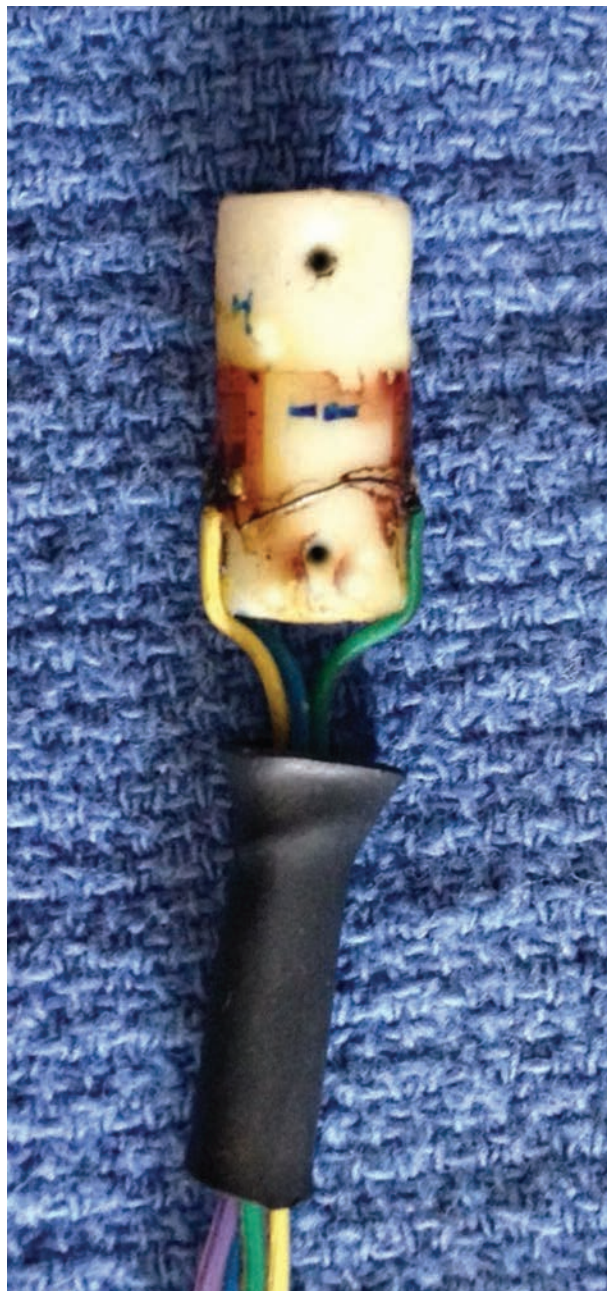
Figure 1 —Photograph of a custom-made transducer for measuring load on the sutures of LTF constructs in horse cadavers used in the study to compare the mechanical properties of LTF constructs prepared with different suture materials and suture placement patterns during single load to failure testing. The miniature 0° to 90° 350-Ω transducer class strain gauge rosettes and short jumper wires are bonded to the central arm with cyanoacrylate adhesive. Notice the heat shrink tubing to protect the electrical connections and the holes drilled in each end of the transducer to allow passage of the sutures.
