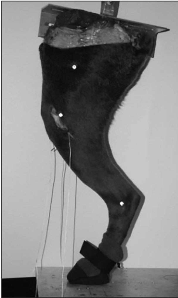
Figure 2—Photograph of a hemipelvis collected from a clinically normal nonchondrodystrophic dog and mounted on a modified OKR for use in a study to quantify the 3-D kinematics and collateral ligament strain of stifle joints in canine cadavers before and after CrCL transection followed by TKR involving various TPAs and spacer thicknesses. The paw is attached rigidly to a platform, and an angle iron is bolted through the ischial tuberosity and sacroiliac joint of the ilium.
