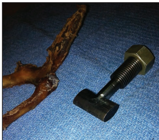
Figure 4—Photograph of an equine basihyoid bone and a custom-made steel model basihyoid bone fixture. Notice that the short transverse bar of the model fixture is oval, whereas the base of the lingual process in the basihyoid bone is round. The horizontal portion of the fixture had a 26-mm-long oval cross-section and was 6.3 mm in diameter horizontally and 12 mm in diameter vertically. The width of the horizontal portion of the steel model basihyoid bone fixture was identical to the distance between right and left basihyoid-ceratothyoid bone articulations in an equine cadaver examined during design of the fixture.
