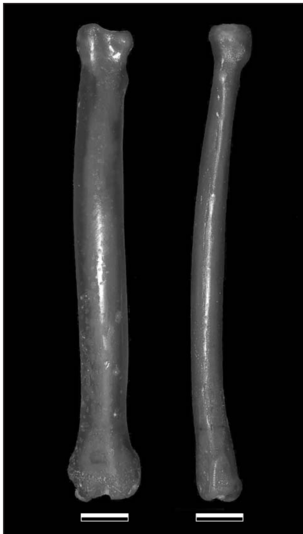
Figure 2—Photograph of the cranial and lateral aspects of a 50% FRC replica of a canine radius. The epoxy-glass fiber mixture (in this instance, the fiberglass-to-epoxy ratio [wt/wt] was 50%) is transparent and free of visible bubbles. The replica length is 205 mm. Scale bars measure 20 mm.
