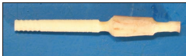
Figure 1—Photograph of an allogeneic bone screw (dimensions, 4.5 \times 40.0 mm) prepared by use of a commercially available precision desktop microlathe programmed with the dimensions of a stainless steel surgical screw. The source of bone material was the dorsal midshaft cortex of the third metacarpal bone from the cadaver of a 3-year-old male Thoroughbred.
