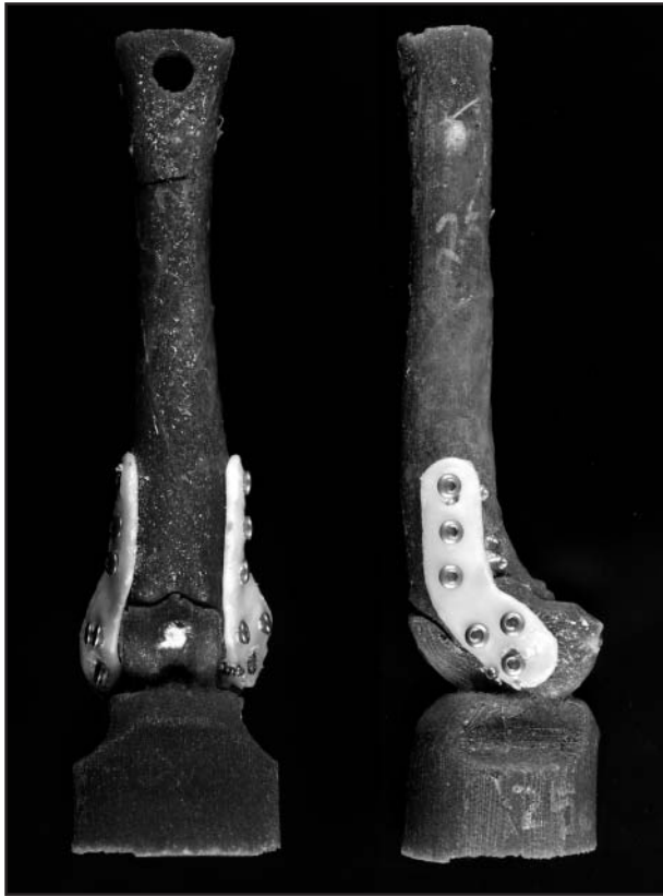
Figure 6—Photograph of the cranial (left) and lateral (right) aspects of a canine femoral replica stabilized by use of two 2-mm-thick PCL bioresorbable plates. Each plate is secured with six 3.5-mm titanium cortical bone screws.
