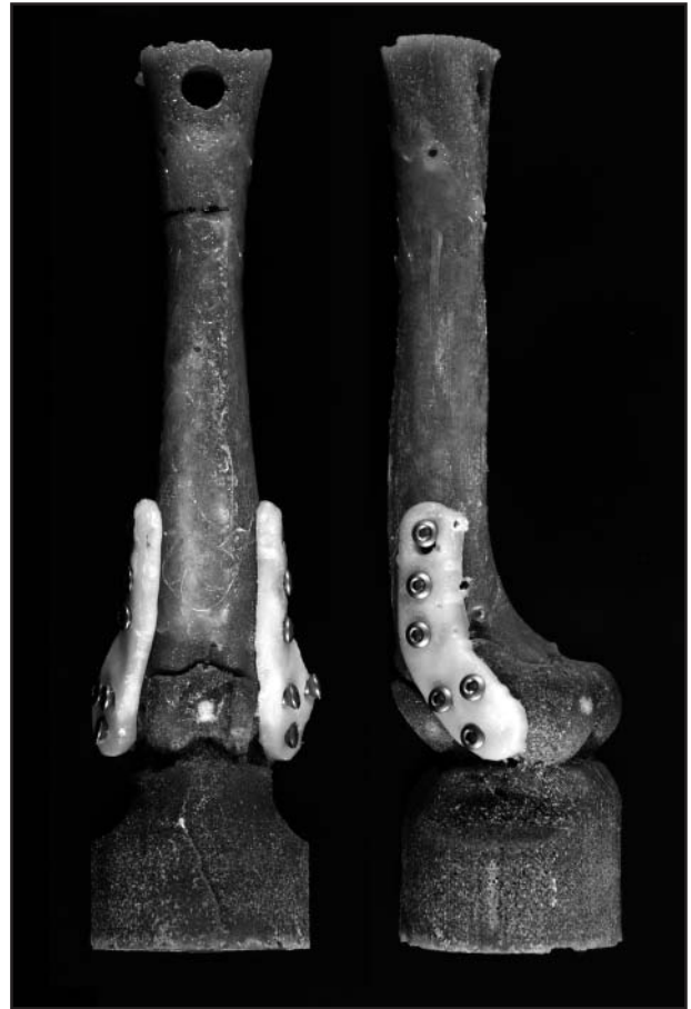
Figure 7—Photograph of the cranial (left) and lateral (right) aspects of a canine femoral replica stabilized by use of two 4-mm-thick PCL bioresorbable plates. Each plate is secured with six 3.5-mm titanium cortical bone screws.
