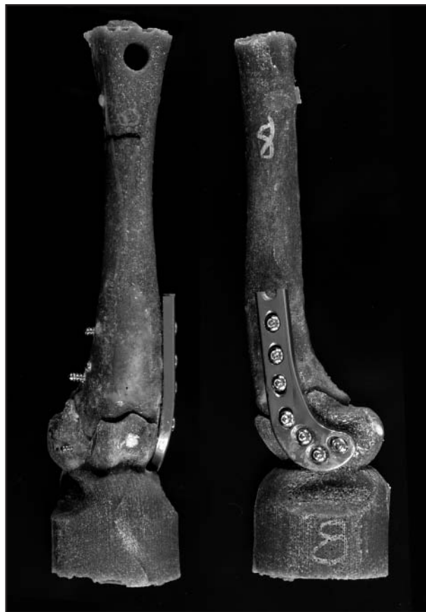
Figure 9—Photograph of the cranial (left) and lateral (right) aspects of a canine femoral replica stabilized by use of a CSP and 7 stainless steel 3.5-mm cortical bone screws. The plate has been contoured to approximate the surface of the bone and has been cut at its proximal aspect.
