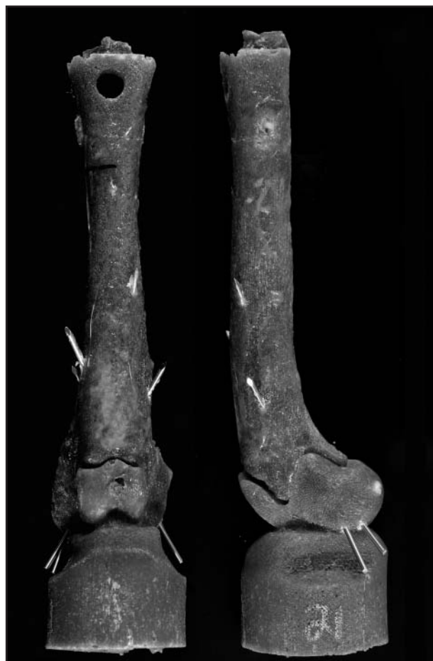
Figure 5—Photograph of the cranial (left) and lateral (right) aspects of a canine femoral replica stabilized by use of four 2-mm-diameter stainless steel Kirschner wires. The wires were placed in a distal to proximal direction and protrude through the near and far cortices.
