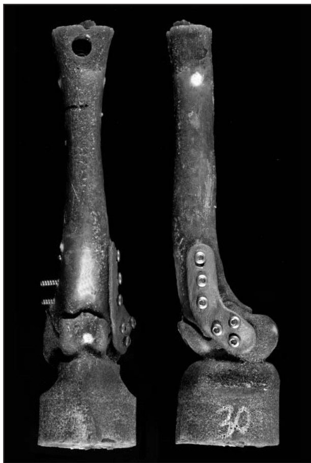
Figure 8—Photograph of the cranial (left) and lateral (right) aspects of a canine femoral replica stabilized by use of a CTP and 6 titanium 3.5-mm cortical bone screws.
