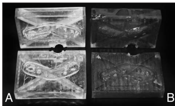
Figure 4—Photographs of injection molds used for fabrication of bioresorbable PCL plates. The molds are made of epoxy-based photopolymer fabricated by use of stereolithography (A) and reinforced with liquid steel epoxy (B).
