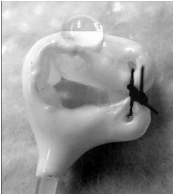
Figure 4—Photograph of an HO5 with a small leak and associated bubble of saline (0.9% NaCl) solution along the seam of the inflatable balloon that was detected during leak testing.
