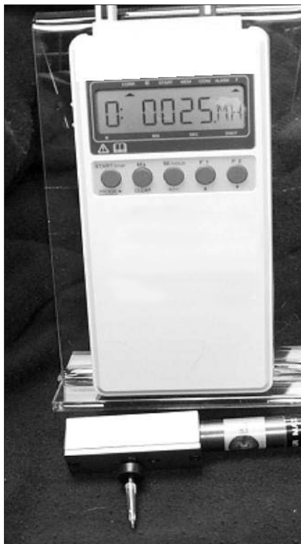
Figure 1—Photograph of a von Frey device with a load cell built into the handle and the tip used to evaluate the antinociceptive effects of morphine in dogs.
