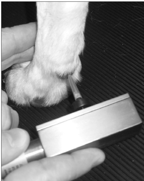
Figure 2—Photograph of the application of the von Frey device to the left carpal pad of a dog.
