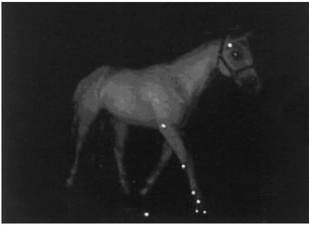
Figure 3—Field of view of camera 1 (frontolateral view; left) and camera 2 (lateral view; right) from Figure 2. The laboratory was darkened to increase contrast between markers, horse, and environment. Reflective markers were illuminated by halogen lamps positioned behind each camera.
