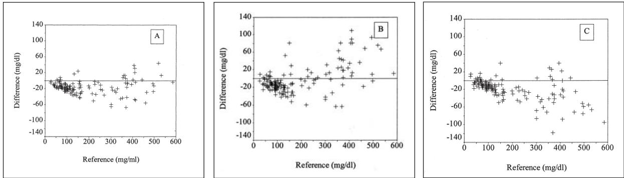
Figure 2—Scatterplots of the differences between blood glucose concentrations obtained by use of a PBGM versus concentration (A, Glucometer Elite; B, Glucometer DEX; C, SureStep; D, Precision QID; E, Accu-Chek Simplicity) obtained with a hexokinase reference method for blood samples obtained from 150 cats.
