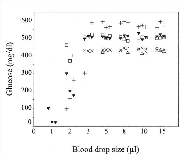
Figure 1—Effect of blood drop size on results of 5 portable blood glucose meters (PBGM; ▼ = Glucometer Elite, + = Glucometer DEX, x = SureStep, △ = Precision QID, □ = Accu-Chek Simplicity) used to measure glucose concentrations in cats.
